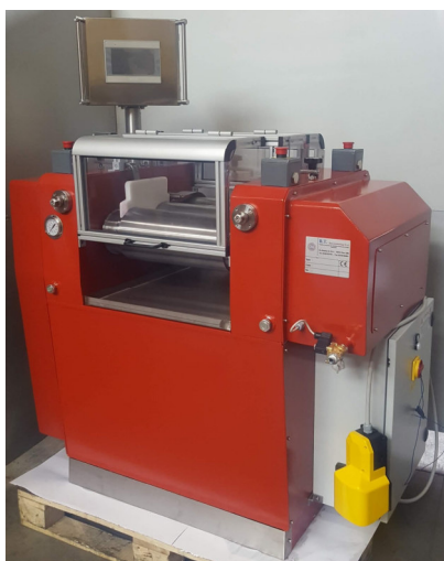
Machine with horizontal cylinders arrangements
